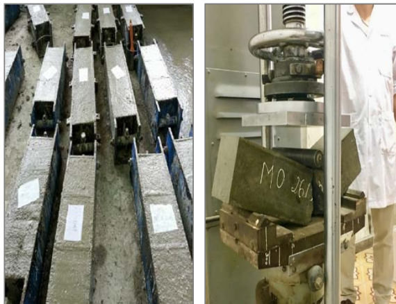
Fig. 5. Sampling and testing of flexural strength
