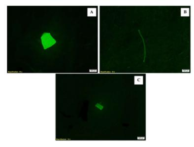
**Figure 5.** At 100x magnification, the microplastic (A) has a length of 229.49  $\mu$ m; fibrous (B) with a length of 524.68  $\mu$ m and granular (C) with a length of 113.81  $\mu$ m.
